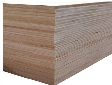
Blockboard is made of wooden strips or block, placed edge to edge between two layers of plywood. It is then glued together under high pressure.
