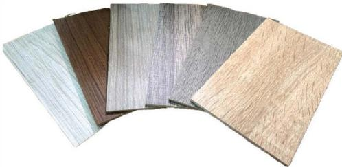
PVC laminated plywood are multi-layered laminate sheets based on Poly Vinyl Chloride. It is made by compressing paper and plastics resins under high pressure and temperature. It comes in a variety of colours and textures and better durability.
