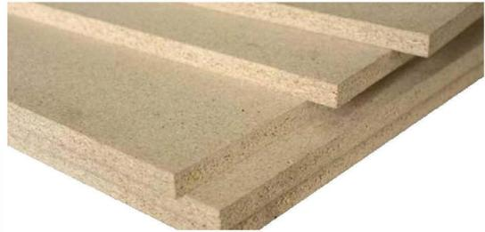
Particleboards are commonly used as coverage for hardwood floors. It is used to prevent hardwood boards from scratches. It is also widely used to make floors in temporary structures.
