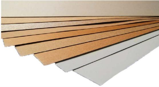
Chipboard is made from reconstituted wood. The material is often shavings, chips or sawdust. It is then compressed and held together using natural or synthetic resin and then formed into boards. .
